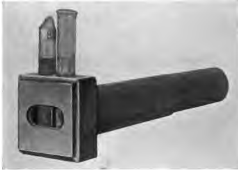
Fig. 92.—The nephelometer; an instrument used for standardizing bacterial suspensions used for the opsonic test or for vaccines, by comparison with precipitate of barium sulphate.
